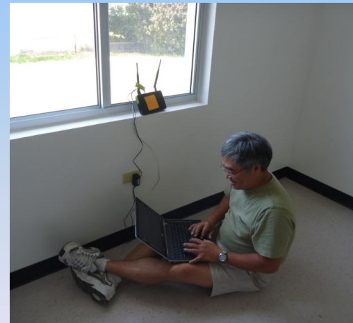
Setup wireless connection repeater for DAWR's fishery new building in April 2013. Wireless signal is captured from adjacent Wildlife building.
