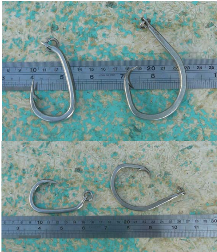
Figure 2. Dimensions of tuna (left) hook and circle hooks (right)
